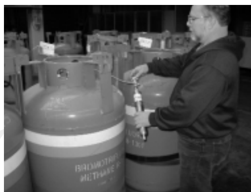
Technician taking a sample of Halon 1301. Recycled halon should be tested by an independent laboratory to ensure product conformance to specifications. Photo courtesy of U.S. DOD/DLA ODS Reserve.
