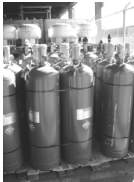
Halon 1301 total flooding system cylinders held in storage. Cylinders such as these are collected from decommissioned systems, and the halon is recycled and banked for critical government and industry programs. Photo courtesy of U.S. Department of Defense (DOD), Defense Logistics Agency (DLA), Ozone Depleting Substance (ODS) Reserve.
