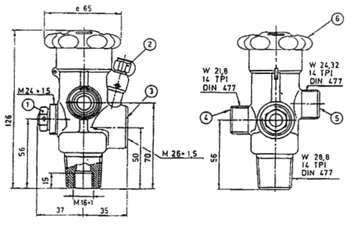
Valve for H1301 High Pressure Cylinder.
