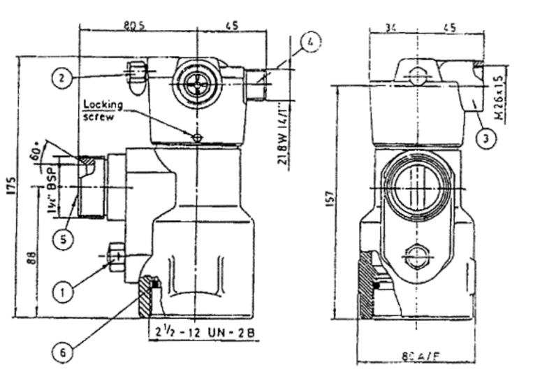
Valve for H1301 High Pressure Cylinder.
