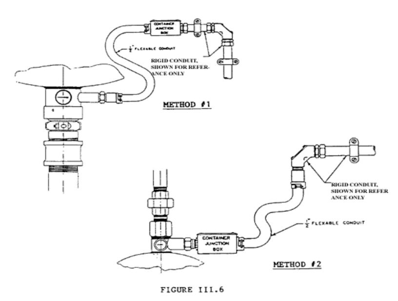
The container must have an agent release module, which is supplied. The agent release module is mounted in the container junction box by means of an adhesive strip located on the back of the module. Do not mount the A.R.M. to the junction box lid.
