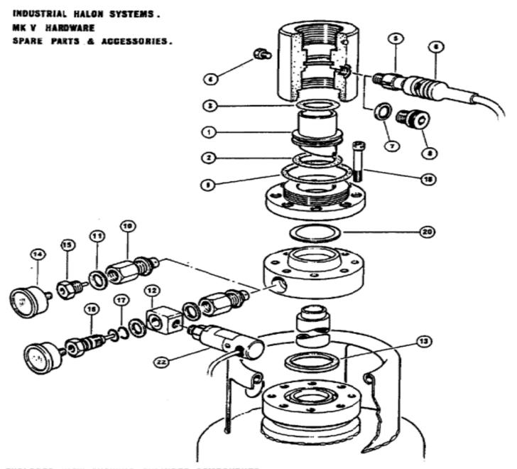
EXPLODED VIEW SHOWING CYLINDER COMPONENTS DISCHARGE HEAD & ALTERNATIVE PRESSURE GAUGE ASSEMBLIES WITH & WITHOUT PRESSURE SWITCH.
